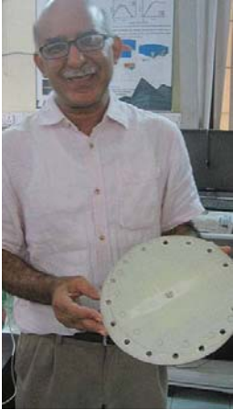
Professor Puneet Mahajan, Applied Mechanics, IIT-Delhi with an experimental plate whose centre has a bullet entry, following a test for the ballistic helmet.
